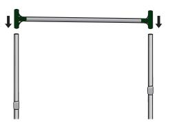
Place the Top Cross Bar previously set aside into each end of tube to be used as the top cross bar.
