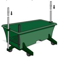
Slide straight connectors into the vertical tubes.
