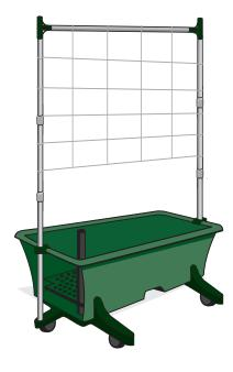
Hang netting over top T-connectors. Tie netting to top tube at equal intervals. Tie netting to vertical tubes at even intervals, starting at the top and working down.
