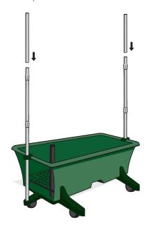
Insert two tubes vertically onto top end of straight connectors.
