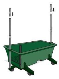
Slide straight connectors into the vertical tubes.
