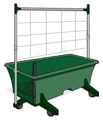
Hang netting over top T-connectors. Tie netting to top tube at equal intervals. Tie netting to vertical tubes at even intervals, starting at the top and working down.
