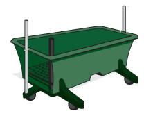
Tubes are identical in length. Insert a tube through the clip and into the outrigger. Repeat for the clip on the opposite end of the box.
