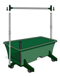
Slide T-Connector & Horizontal Bar assembly into Vertical Tubes.
