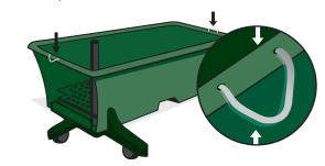
Insert the clips through the holes drilled through the rim at each end of the EarthBox.
