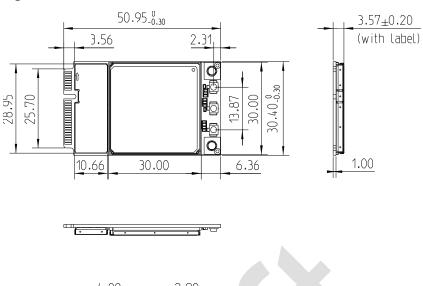
Figure 6-1 Dimensions of the MC509 module
