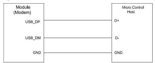
Figure 3-9 Recommended circuit of USB interface
