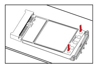
Step 3 Use a screwdriver to fix the Mini PCle Adapter on the main board with two screws provided in the Mini PCle Adapter packing box.
