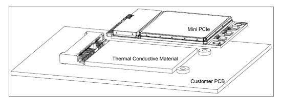
On the customer PCB, reserve two metal screw holes, which are connected to the PCB ground plane. When installing the Mini PCle, use two metal screws to fasten the Mini PCle to the customer PCB. See the following figure.
