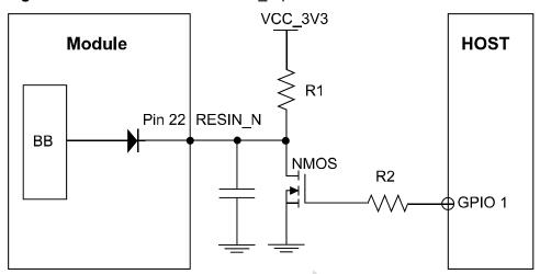
Figure 3-5 Connections of the RESIN N pin
