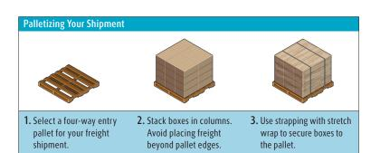
Pallets with four-way forklift entry are preferred as they help to improve handling and reduce damage to the shipment
