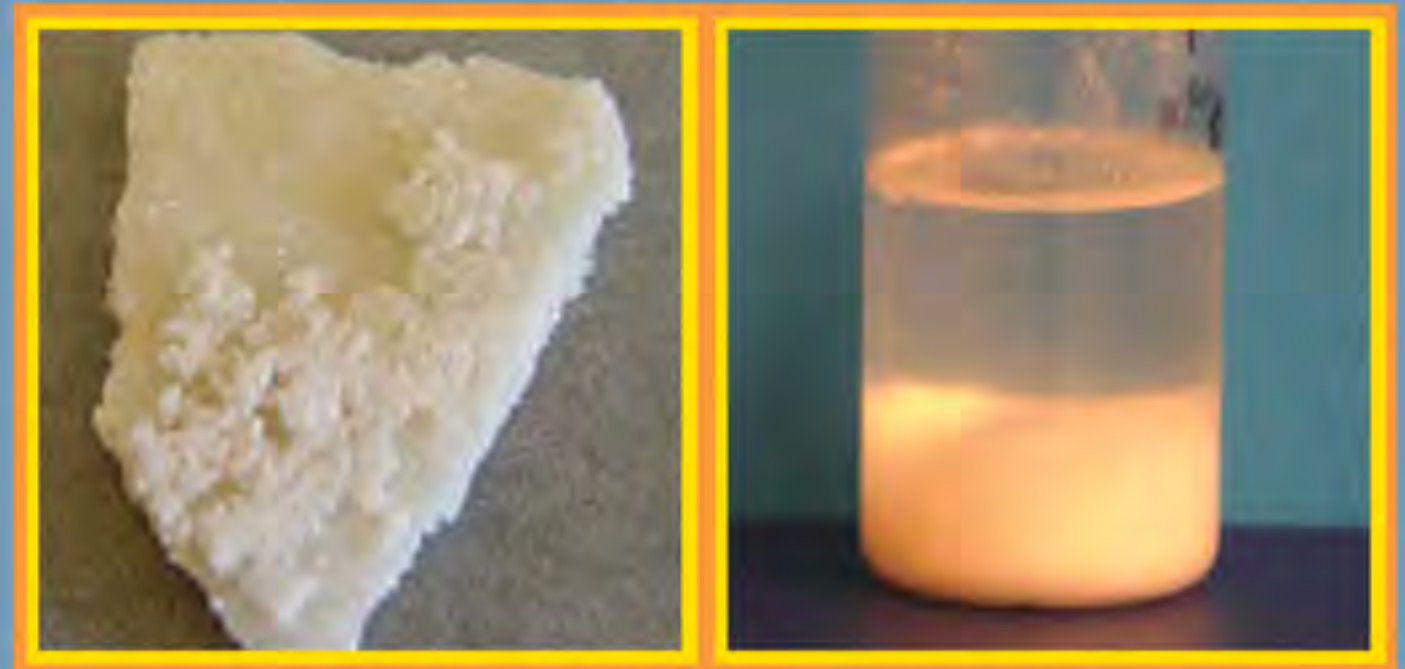
Chemical Disintegration of \text{CaSO}_4 Scale
