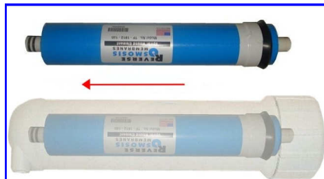
Insert the RO membrane into housing, 2 black rings go in first
