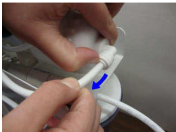
Remove tube and cap from RO housing
