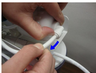
Remove tube and cap from RO housing
