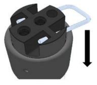
Step 3: Use U-pin as a pry tool to leverage out hub
